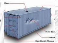
We found that built out SeaCans sustain significant damage and/or lose parts of the assembly - i.e. propane for hvac, tooling for specialty applications, gensets etc.
